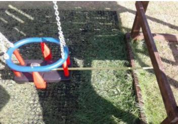
**Finding:** The surfacing width under each seat is less than 1.75 metres and fails the requirements of BS EN 1176 Part 2
