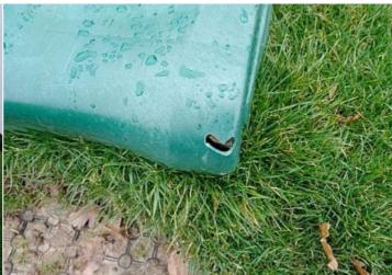
Finding: The run out section of the slide has been damaged Action: Repair or replace the item
